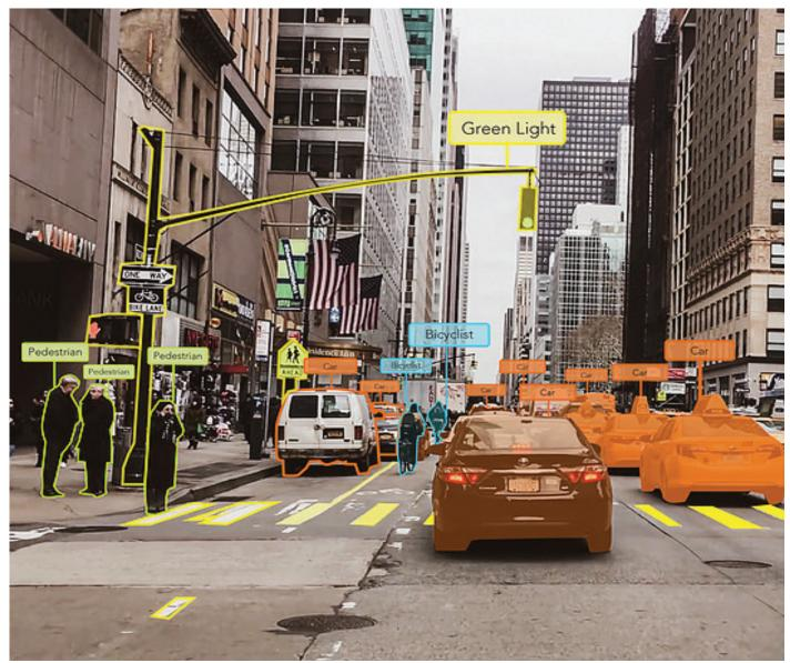
Cameras mounted on city buses and other municipal vehicles have the ability to detect vehicles, traffic lanes, lights, and pedestrians among other features. Technology allows for these cameras to help with traffic enforcement - such as illegally parked cars or cars parked in bus lanes - and can help map city infrastructure, reserve curbs for delivery, use data to determine the best traffic patterns to ease congestion, and speed up travel times in communities.
